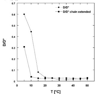
**Figure 3.**Normalized diffusion coefficient as function of temperature for or commercial and chain extended Pluronic F127. The values of diffusion in F127 had been normalized respect the data in water in order to decouple the effect of beads diffusion in the solvent of solution.
